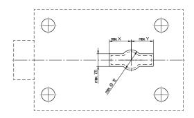
Fig. 3: Max. cross sectional area of keyhole
