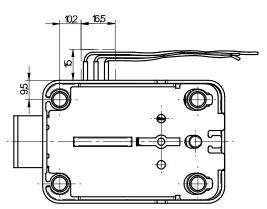
Fig 5: Keep clear area for cables
