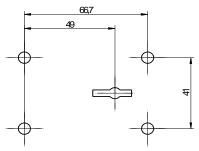
Fig. 4: Fastening hole pattern
