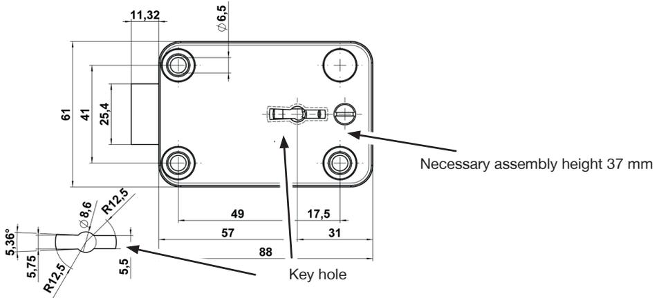
The ease of movement of the bolt in locking mode must be guaranteed. When using bars, angles or similar blocking elements attached to the bolt, transverse forces, resp. friction on the lock bolt must be avoided through construction measures. The lock has been tested with an actuating force of 2.5 N.
