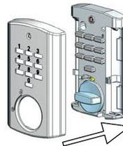
After the cover has been installed, the key tones will sound deeper until a valid code has been entered. If, despite the correct mounting of the cover, you hear deep tones, check the keyboard for possible tampering!
