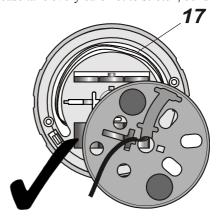
the bottom plate back in place. This completes preparing the input unit for mounting. When fitting the bottom plate, make absolutely sure not to pinch or otherwise damage the strands of the keyboard cable. Even minor damage to the strands during assembly may eventually cause the cable to break.
