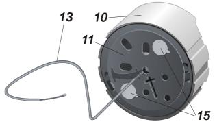
The input unit has two pinning positions; one is for mounting electromechanical lock module (1) vertically, the other for mounting electromechanical lock module (1) horizontally.
