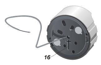
B) To mount the lock module horizontally, use the second pin position, thus causing the locking pin to be entered vertically from below. To gain access to the required pin entering slot, turn the bottom plate until the cross-shaped through-hole (16) is vertical, below, when looking on to the bottom plate. The spindle connection is pinned and secured in this position as described for the first mounting variant,
