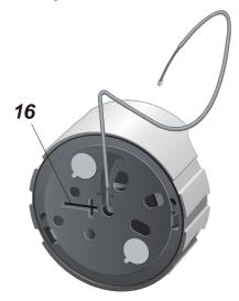
A) If the lock module is to be mounted vertically, as shown in the first diagram, the pin hole is horizontal and the first horizontal pinning position has to be used. After checking that the input unit is locked in place, turn the movable bottom plate until the cross-shaped through-hole (16) is horizontal on
