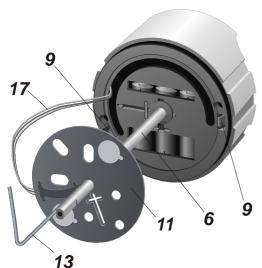
are fixed to the bottom plate and the bottom plate can only be removed by the amount of freedom provided by the loop into which the cable strands have been shaped. Please take every care not to stretch, bend
