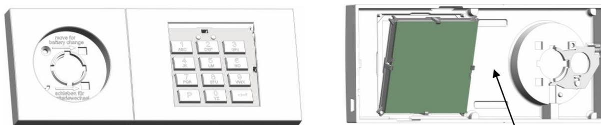
**Figure 40: After removing the top holder, turn around the fitting**
